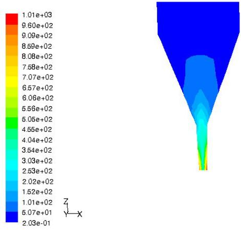
**Figure 6: Contours of the turbulence kinetic energy ( $m^2/s^2$ ) at a cross section located at the centre of the air-knife body**
