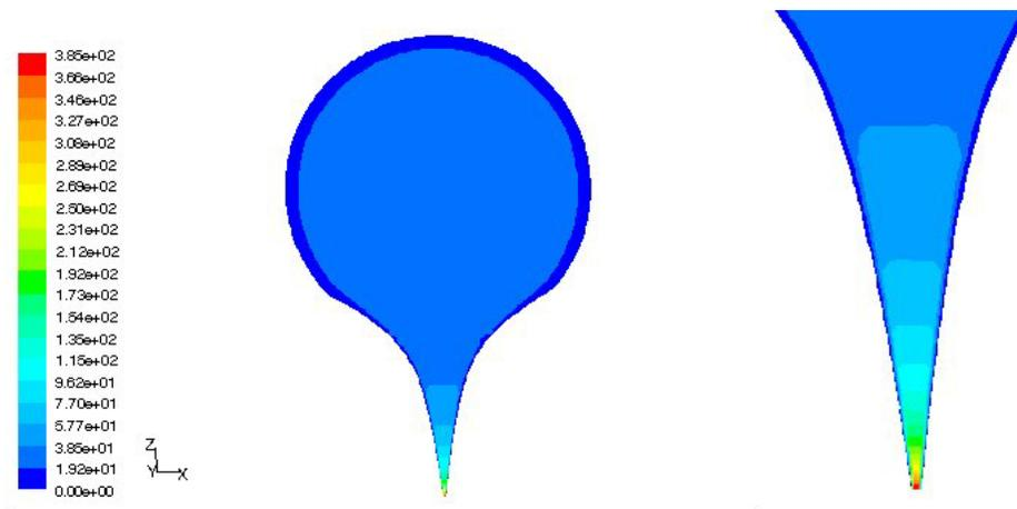
**Figure 9: Contours of the velocity magnitude (m/s) for a cross section located at the centre of the air-knife body**
