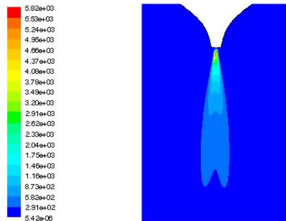
Figure 16: Contours of the turbulence kinetic energy ( $m^2/s^2$ ) around and downstream of the exit of the nozzle, for longer domain
