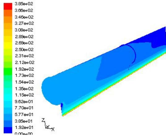
**Figure 10: Contours of the turbulence kinetic energy ( $m^2/s^2$ )**
