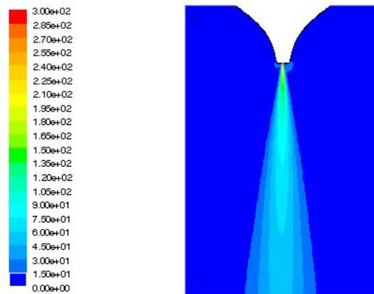
Figure 15: Contours of the velocity magnitude (m/s) downstream of the exit of the nozzle, for the proposed external shape
