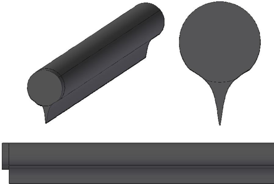
**Figure 8: Proposed internal domain of the air-knife body**
