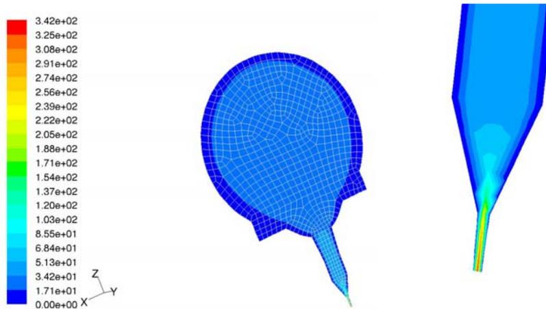
**Figure 5: a) Contours of the velocity magnitude (m/s) at a cross section located at 0.5 m from the exit and the plane mesh. b) Detail of the contours of the velocity magnitude at the exit of the nozzle**
