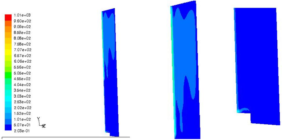
**Figure 7: a) Contours of the turbulence kinetic energy ( $m^2/s^2$ ) at a centre plane of the air-knife body b) Detail of the close end of the body c) Detail of the open end of the body**
