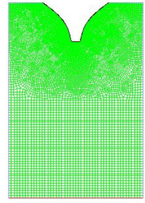
Figure 14: Plane mesh at the external part of the nozzle, for the proposed geometry
