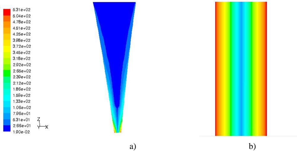
**Figure 11: Contours of the turbulence kinetic energy ( $m^2/s^2$ ) at a cross section located at the centre of the air-knife body a) Detail at the bottom of the geometry, at the exit of the nozzle**
