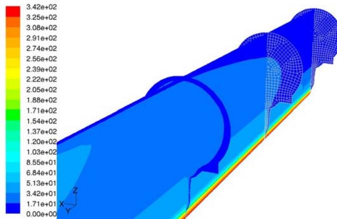
Figure 4: Contours of the velocity magnitude (m/s) for three different cross sections combined with a centre plane of the air-knife
