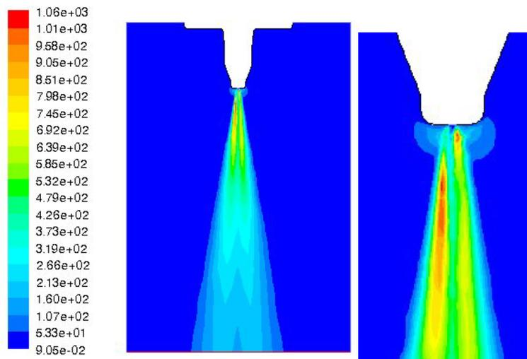
**Figure 13: Contours of the turbulence kinetic energy ( $m^2/s^2$ ) around and downstream of the exit of the nozzle, for longer domain**
