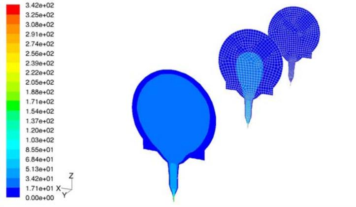
Figure 3: Contours of the velocity magnitude (m/s) for three different cross sections
